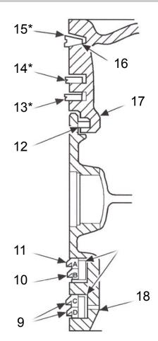
\* Align gaps of 1st and 3rd rings 180 degrees from gap of 2nd ring
